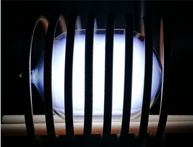
Fig. 7. Lamp in stabilized operation at 3.026 MHz and 150 W.
