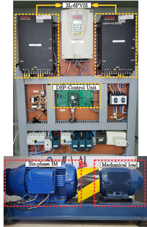
Fig. 8. Test bench composed of the 2L-6PVSI, DSP unit control, six-phase IM, and the mechanical load.
