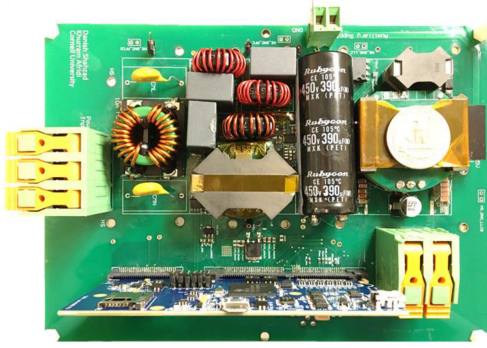
Fig. 20. Photograph of the prototype 1-kW universal input to 28-V isolated soft-switched ac-dc converter, which achieves a power density of 84 W/in 3 (5.13 mW/mm 3 ).
