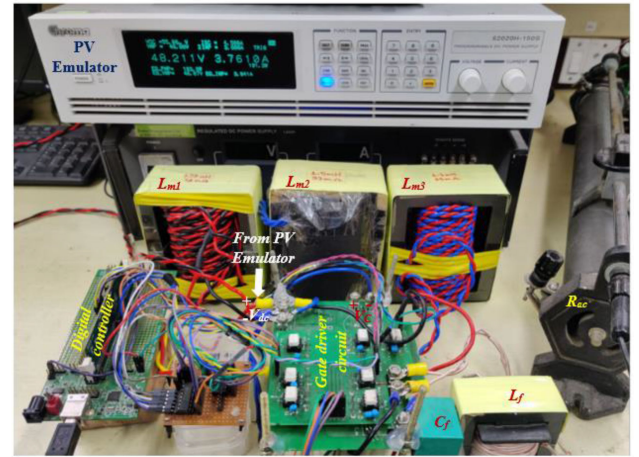
Fig. 16. Experimental prototype of a two-phase ICCFT.
