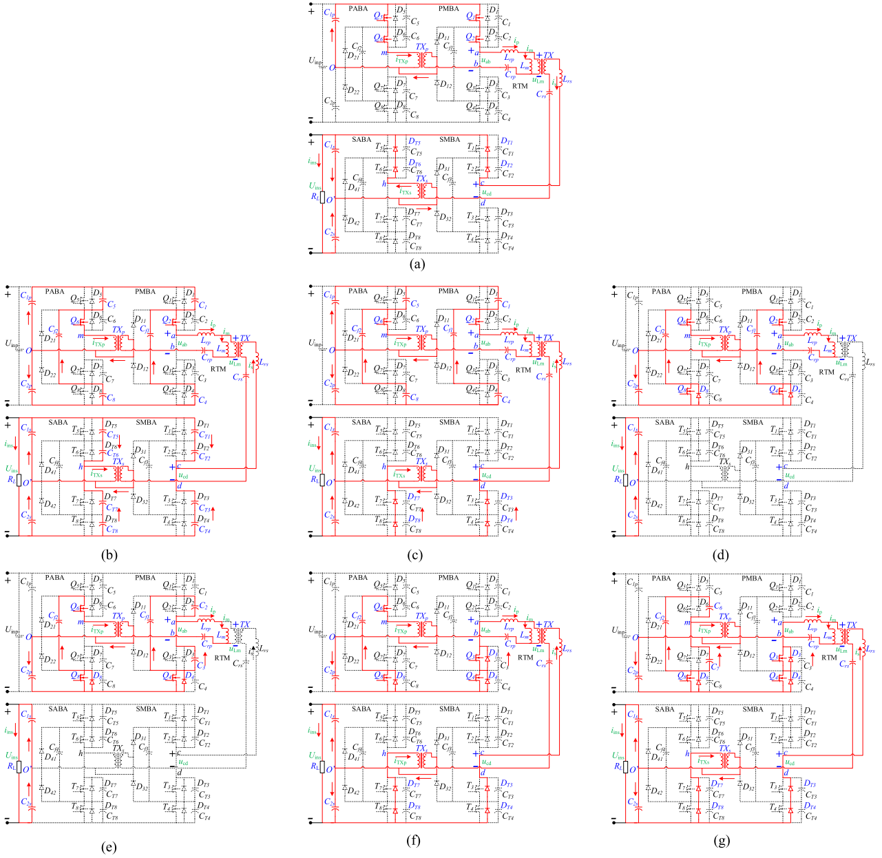
Fig. 3. Key states of equivalent circuits to MVGM. (a) State I [ t_0, t_1 ]. (b) State II [ t_1, t_1' ]. (c) State II [ t_1', t_2 ]. (d) State III [ t_2, t_3 ]. (e) State IV [ t_3, t_4 ]. (f) State V [ t_4, t_5 ], and (g) State VI [ t_5, t_6 ].
