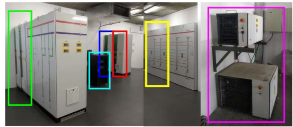
Fig. 9. Lab photograph. From left to right: (green) 75 kVA converter used as emulator for the SG and part of the load in MG1, (cyan) real-time targets (converter controllers), (blue) 15 kVA converter used as GFo-VSC, (red) 15 kVA converter used as GFe-VSC, (yellow) ac bus bars and (magenta) loads.
