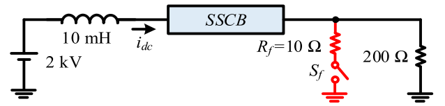
Fig. 7. Simulated circuit in LTspice to emulate a short circuit interruption.
