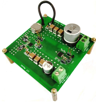
Fig. 19. Prototype of the GaN-based buck converter. Parameter set of this prototype is given in Table I. It is a prototype of the circuits shown in Figs. 6, 7, 9, and 10.
