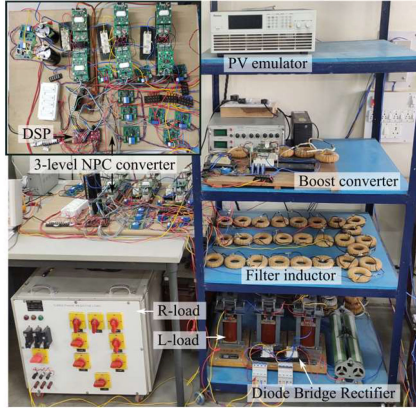
Fig. 9. Experimental setup for implementing the SVHCC technique for the three-level NPC inverter for DG and SAPF application.
