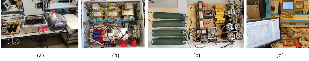
Fig. 4. Test bench: (a) VSI and LC filter, (b) LC filter and voltage and current sensors, (c) nonlinear load and, (d) control hardware and user interface.
