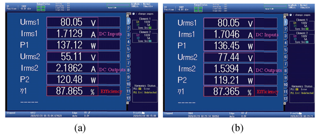
Fig. 19. Screen capture of power analyzer at (a) start and (b) end of the charging process.
