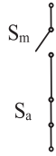
Fig. 4. SC configuration to guarantee that the failures of the main switch S_m always lead to an open circuit, by opening the auxiliary switch S_a , which performs the function of an electronic fuse [27].
