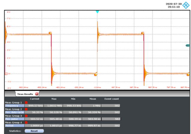
Fig. 17. Measured voltage at the output of LMG5200 half bridge.
