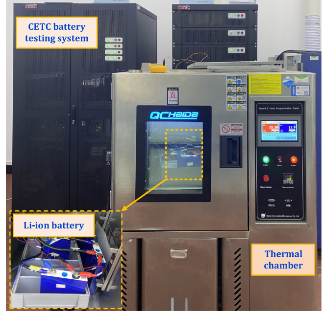
Fig. 6. Battery testing platform.
