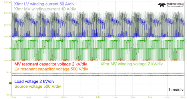
Fig. 20. Single-module experimental waveforms at about 2 kV, 10 kW of the modular soft-switching solid-state transformer (M-S4T) prototype.
