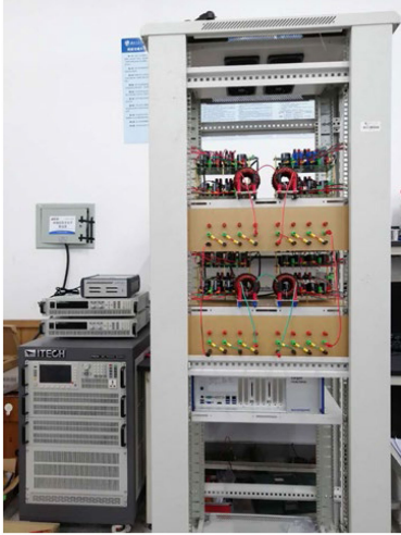
Fig. 12. Downscaled laboratory prototype of MMC.
