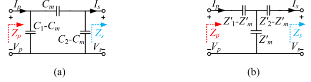
Fig. 2. Models of the capacitive coupler. (a) \Pi -type model. (b) T-type model.
