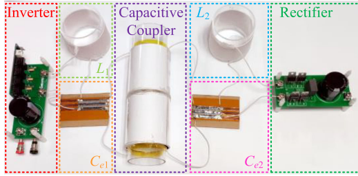
Fig. 17. Experimental prototype of the CPT system.
