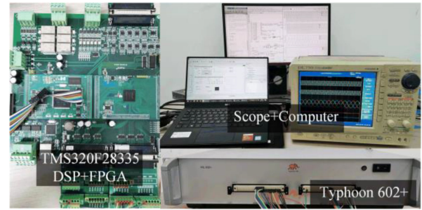
Fig. 15. Hardware platform of CHIL experiment.
