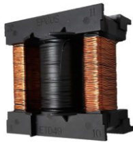
Fig. 24. Variable inductor prototype.
