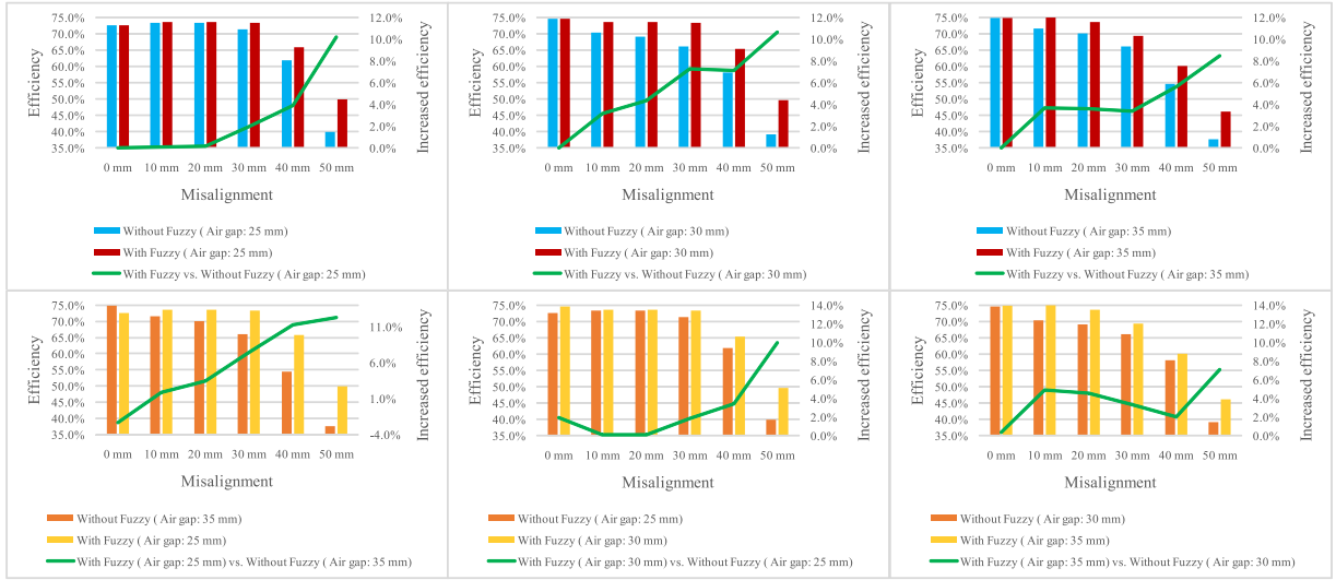
Fig. 38. Trend of power transfer efficiency with respect to coil misalignment and control effectiveness.
