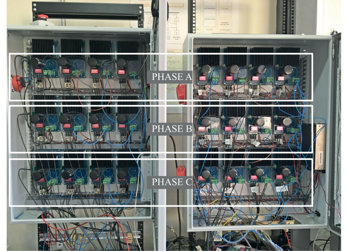
Fig. 8. Experimental setup (left/right cabinet: upper/lower arms).
