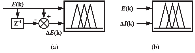
Fig. 10. Different input parameters for the FLC methods. (a) Type 1. (b) Type 2.
