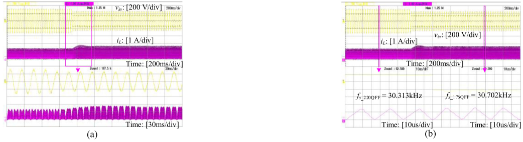
Fig. 23. Transient response of the inductor current with QFF under the input voltage step change between 220 and 176 VAC at 100% load. (a) Around the step change point. (b) In switching cycles during the two stable operation.
