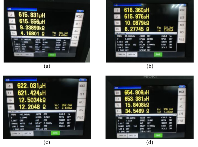
Fig. 30. High-frequency resistance of the inductor with COT measured by the HIOKI IM3536 LCR meter. (a) At 51 kHz. (b) At 65 kHz. (c) At 100 kHz. (d) At 180 kHz.
