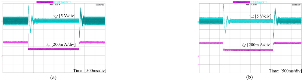
Fig. 25 Transient response of the output voltage with the load step change at 220 VAC. (a) With COT. (b) With QFF.
