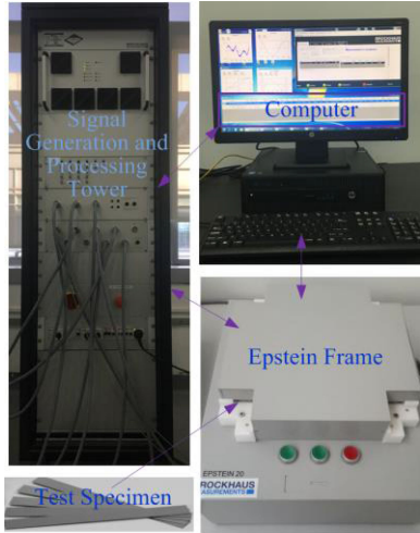
Fig. 3. Brockhaus magnetism measuring apparatus with Epstein frame. The signal generation and processing tower, computer, and the Epstein frame are connecting with each other to conduct the experiment systematically.
