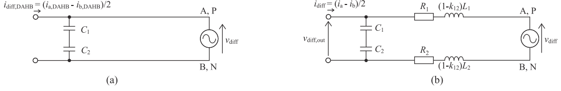
Fig. 5. Equivalent circuit for the differential-mode current of each topology. (a) DAHB converter. (b) Proposed converter.
