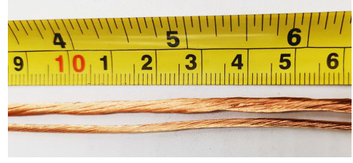
Fig. 5. Litz wires of 1 \times 30 and 5 \times 100 for verification.
