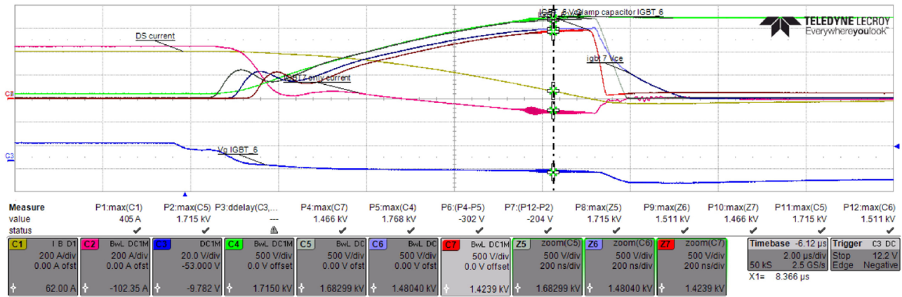
Fig. 5. Random delays in the turn-OFF signals of series-connected IGBTs results in large V_{CE} voltage differences among IGBTs.
