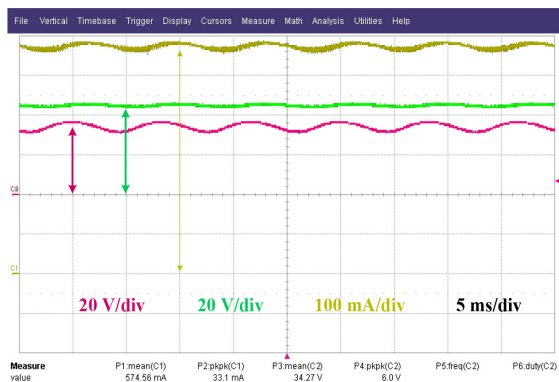
Fig. 13. Bulk voltage (red), output voltage (green), and output current (yellow).
