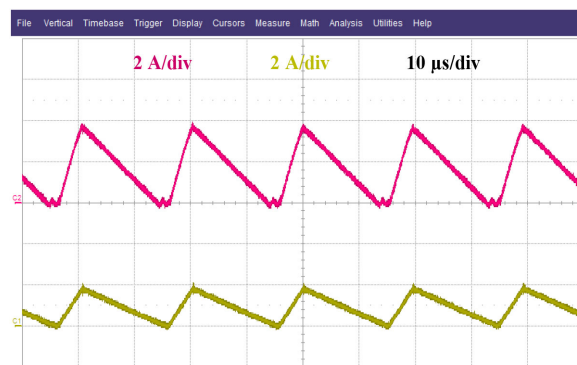
Fig. 16. Buck inductor current (in red), and the boost inductor current (in yellow).
