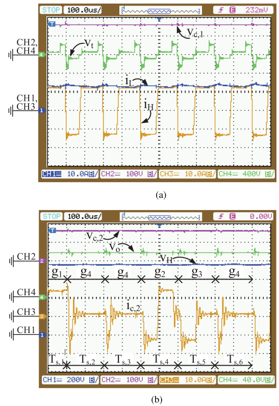
Fig. 10. Steady-state experimental waveforms. (a) v_{c,1} , v_t , i_L , i_H . (b) v_{c,2} , V_H , v_o , i_{c,2} .
