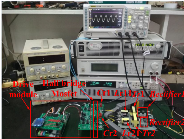
Fig. 19. Test setup picture of prototype with proposed structure.
