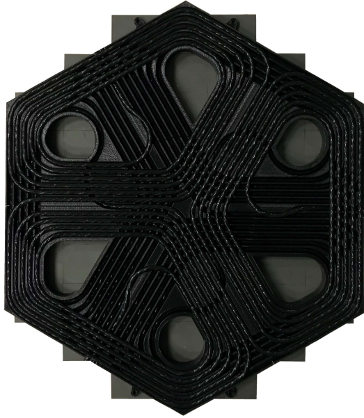
Fig. 13. Two-layer coupler prototype. The bounding box of the pad is 47.1 cm \times 54.4 cm. The total coil mass including ferrite, Litz wire, and wire guides is 13.7 kg. The wire is 6 AWG type 2 Litz with a strand gauge of 38 AWG produced by New England Wire. The ferrite backing is constructed from Ferroxcube PLT64/50/5 tiles of 3C94 material.
