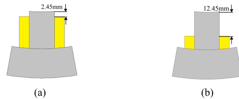
Fig. 21. Two types of winding placement. (a) Type I. (b) Type II.
