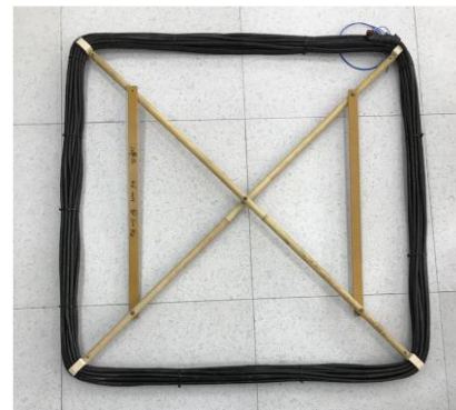
Fig. 11. 1 m \times 1 m, 128 turns loop for the current inverter.
