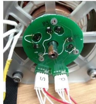
Fig. 15. Six Hall-effect sensors mounted at two PCBs at 30 mechanical degrees apart; the magnetic disc is removed.
