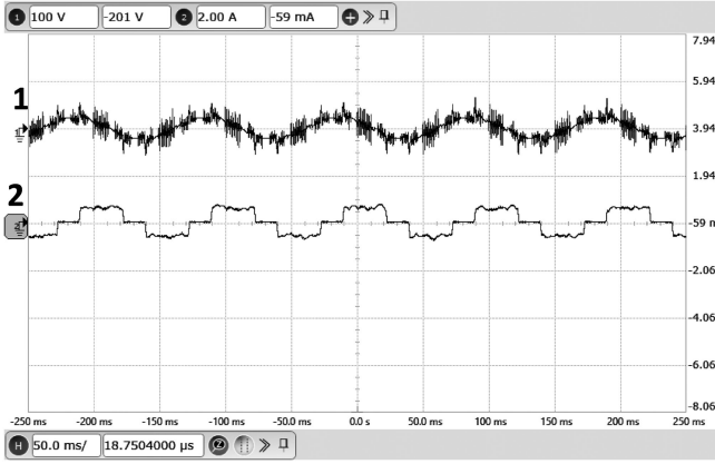
Fig. 21. Experimental results: Motor operation at 300 r/min with single CSI: X-axis: 50 ms/div. Ch-1: Phase-a stator voltage of motor (Y-axis: 100 V/div). Ch-2: Phase-a motor current (Y-axis: 2 A/div).
