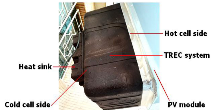
Fig. 5. Photo of the constructed TREC system positioned on the backside of the PV module.
