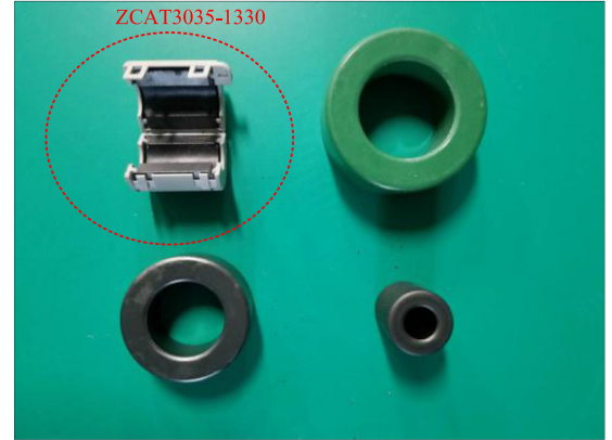
Fig. 12. Several ferrite rings tested in the experiment.
