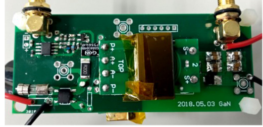
Fig. 10. Test board of the proposed topology.
