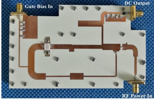
Fig. 11. Photo of the self-driving RF-DC rectifier.
