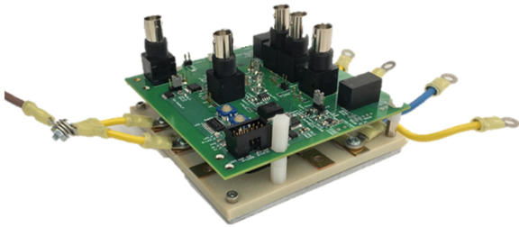
Fig. 15. Fabricated module with a gate drive board.
