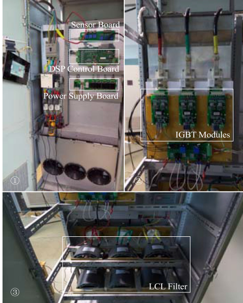
Fig. 9. 30 kVA LCL-type shunt APF prototype in the experiments.
