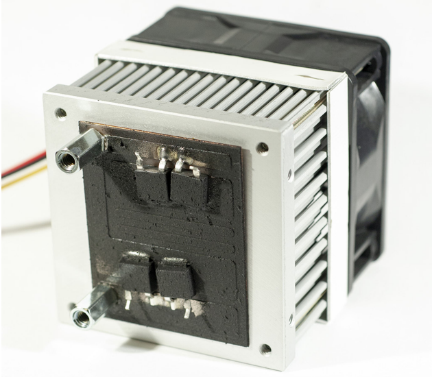
Fig. 15. Multichip thermal test vehicle mounted onto forced-air heatsink and fan.
