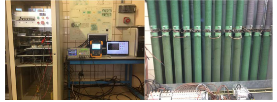
Fig. 6. Laboratory prototype of three-phase three-level NPC power converter.
