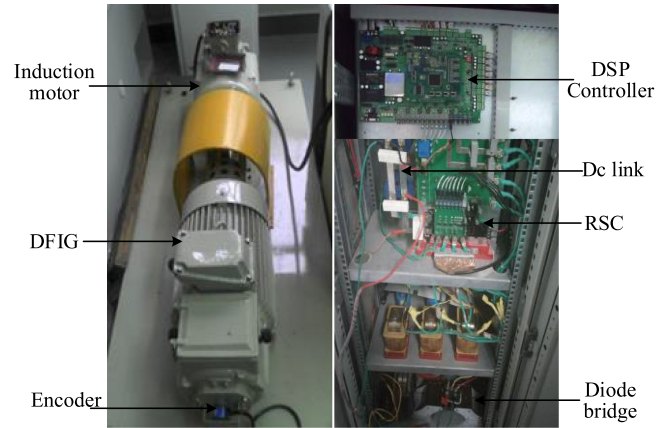
Fig. 17. Experimental setup of the DFIG-DC system.
