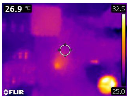
Fig. 9. IR image of the evaluation board top view after 30 min operation.
