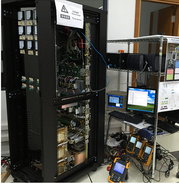
Fig. 13. 110 V-5 kVA SVC-HAPF experimental prototype and its testing environment.
