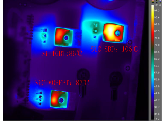
Fig. 14. Infrared images of the hybrid switch at 9 kW.
