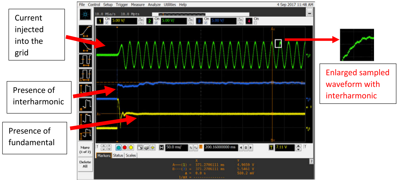
Fig. 10. Current injected into the grid and the signals of the fundamental and interharmonic components (5 V/div for the three traces; 50 ms/div).
