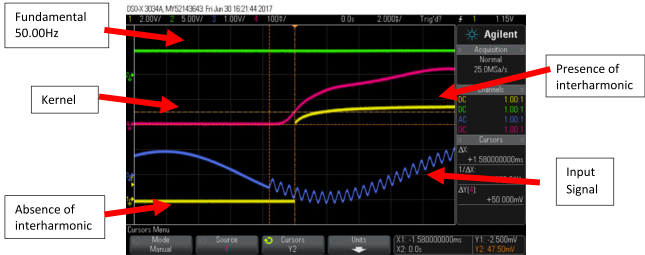
Fig. 8. Practical input signal with fundamental frequency of 50 Hz superimposed with an interharmonic of 1.64 kHz, and the analog versions of the computed fundamental and interharmonic frequency (2 ms/div).
