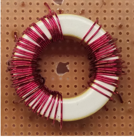
Fig. 12. Five windings' coupled inductor on an iron powder core. On the left side are three well coupled windings and on the right side two well coupled windings. But these last two windings are not so well coupled to the first three ones.
