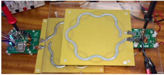
Fig. 33. Photograph of the load-independent synchronous Class E rectifier setup.
