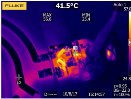
Fig. 22. Thermal steady-state image of the load-independent Class EF inverter at the 150-W input power.
